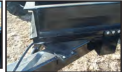
UHMW Wear Plate on Rear Axle
