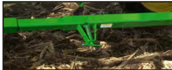
Snap Pin used When Switching Between Transport and Articulation Mode
